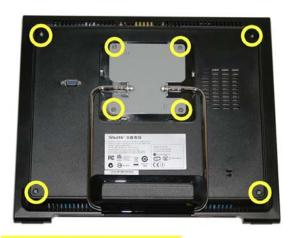
(3) Loosen the four cross-head screws (or Phillips screws) to remove the stand.
