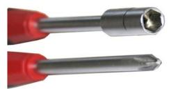
(1) As for tools, one 5mm hexagon screwdriver and one for cross-head screws is required.
