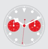
The chronograph function enables you to measure times to fractions of a second, thanks to the centre seconds hand. On some models, to be enabled for use, the pushers must be unscrewed; lock the pushers after use
