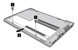
3 Remove the frame fixing screws 3.
